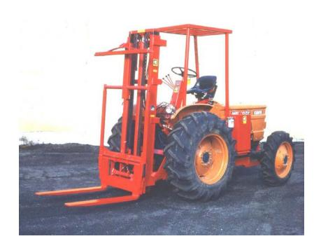
HERE IS THE COMPLETE PACKAGE. THE EDWARDS TRANS-FORK SERIES TF79120S, 4,000 POUND LIFT CAPACITY 120 INCH LIFTING HEIGHT WITH SIDESHIFT, REVERSE STEERING AND OVERHEAD GUARD.
